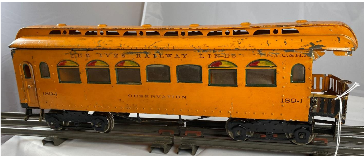
Picture seven is a 1922 passenger car truck with the pickup roller for the light. There is a lever that could hold the roller up (as shown) to turn off the light. That is not present on later trucks. Also note the early Ives coupler held with a cotter pin.
