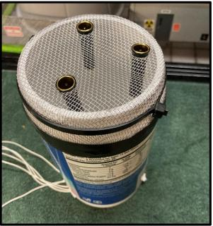
The next step was to fabricate a holder for the smoke units. Now, I am one of those guys that never throws anything away, and from my stash of containers, I found a plastic supplement container that was exactly the right diameter. After cutting the cylinder to the right height, I covered one end with screen wire. I made small slits in the screen wire and pushed in the Sueth smoke units. I had decided to use three smoke units, they produce a genuinely nice stream of steam.
